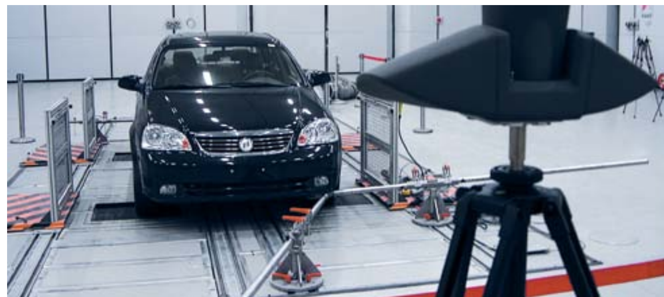
Messhalle für simulierte Vorbeifahrtgeräusch- messung; Tongji University, Shanghai Measurement hall for simulated pass-by noise measurement; Tongji University, Shanghai
