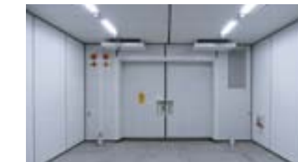
Zwei in einem (Hybridlösung): Klima-Akustik- Kammer; Denso, Eching Two in one (hybrid solution): climatic acoustic chamber; Denso, Eching, Germany
