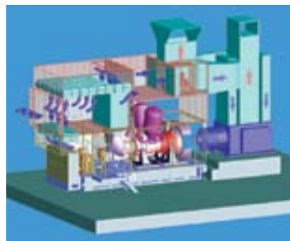
Above: Sound enclosure for transformer station, project E.ON, Germany Left: Noise enclosure and filter house for gas turbine generator set GPB 80 of KAWASAKI Gas Turbine Europe Right: Air flow concept of GT compact package unit MAN Diesel & Turbo SE
