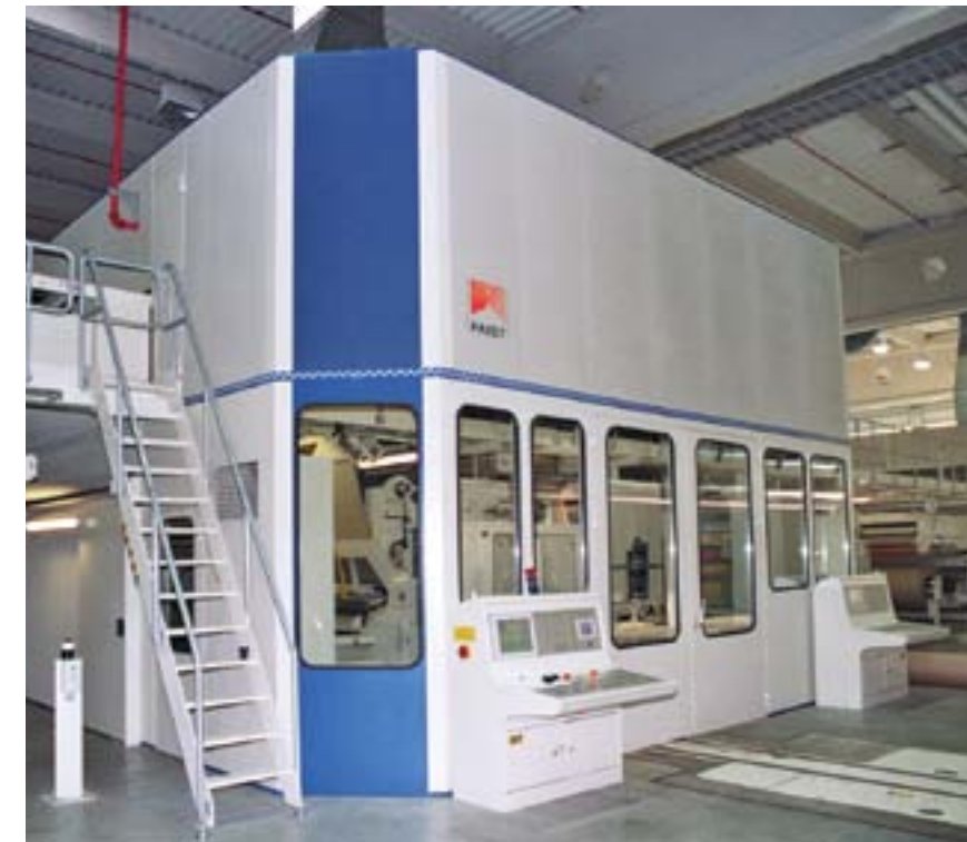
Noise Control for BHS-Modulfacer, Eurowell, Wörth, Germany
