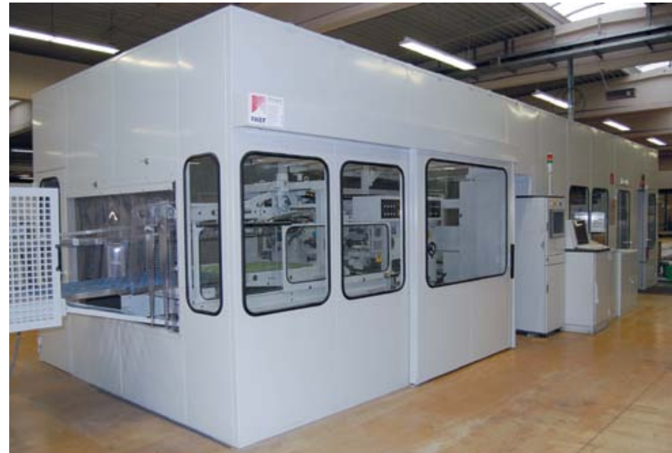
Above: Partial acoustic fencing Mid: Enclosure for Curioni InLine-machine, Kolb, Memmingen, Germany Right: Noise control for Klett InLine-machine
